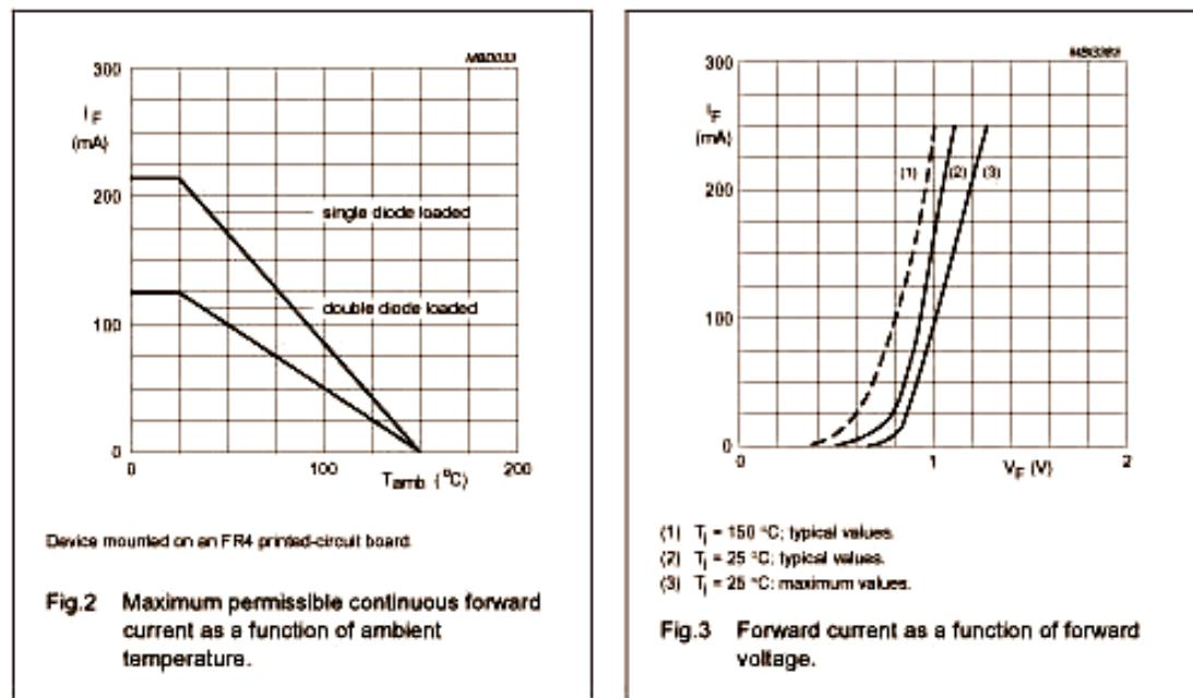
Fig.2 Maximum permissible continuous forward current as a function of ambient temperature.
